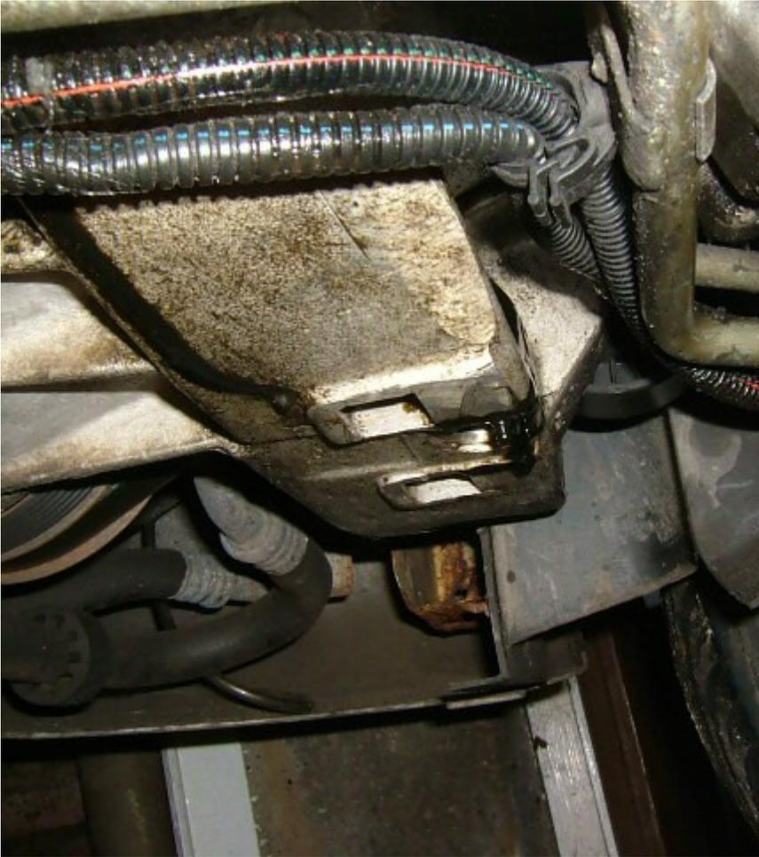
Removing the **filter** by hand can be very tricky or impossible. Due to the **filter** being so short none of the usual wrap-around tools will fit, so get a proper **filter** wrench set (I got a set of 14 from ebay for about £30) and select the correct size like this:
