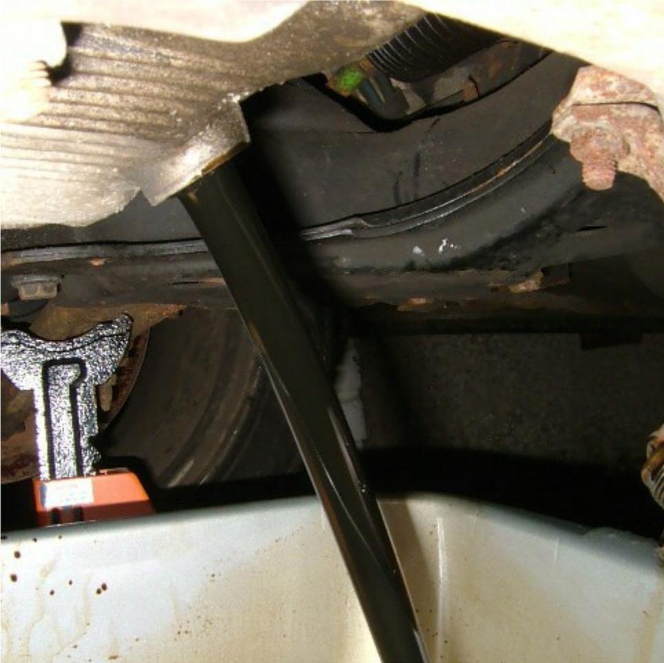
Leave for 10-20 mins to drain into the basin, then put a rag (or small plastic container) under the last of the drips and move the basin forward to catch the rest of the oil when you remove the **filter**, make sure it's under the 2 drain holes shown in the next pic.
