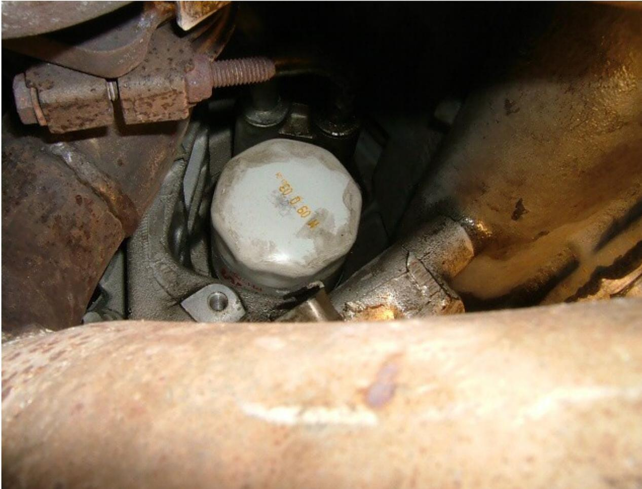
The standard **filter** is very short which makes it even more awkward to fit/remove. There's a suitable Champion **filter** F108 which is a bit **longer** but I couldn't source one of these anywhere locally so got another equivalent which was even **longer**, a Coopers Z68 **filter**.
