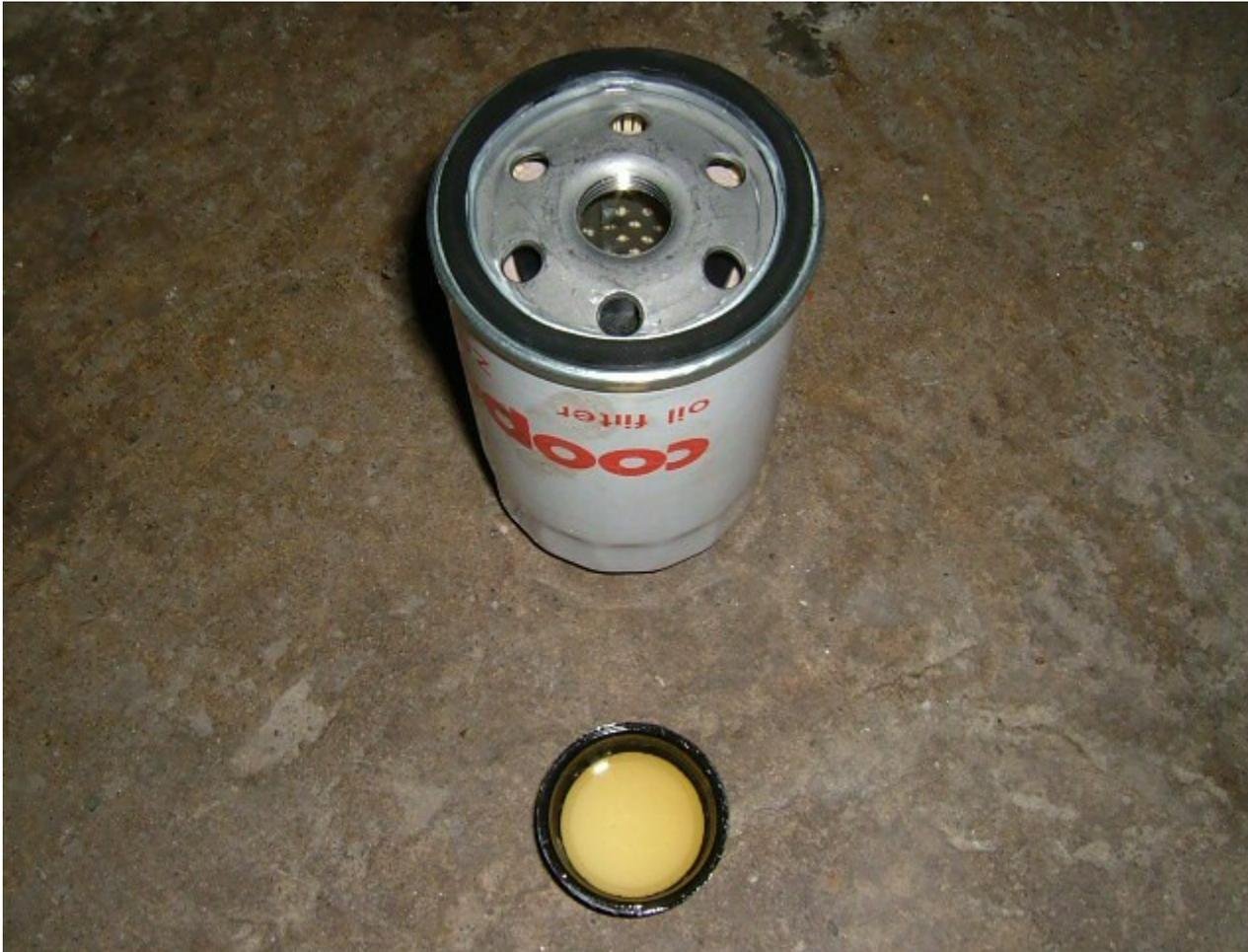
Tighten the new **filter** in place by hand, then use the wrench to give it a final 1/2 turn. The coupe is famous for leaking oil from around the **filter** so make sure it's tight, but don't over-tighten!
