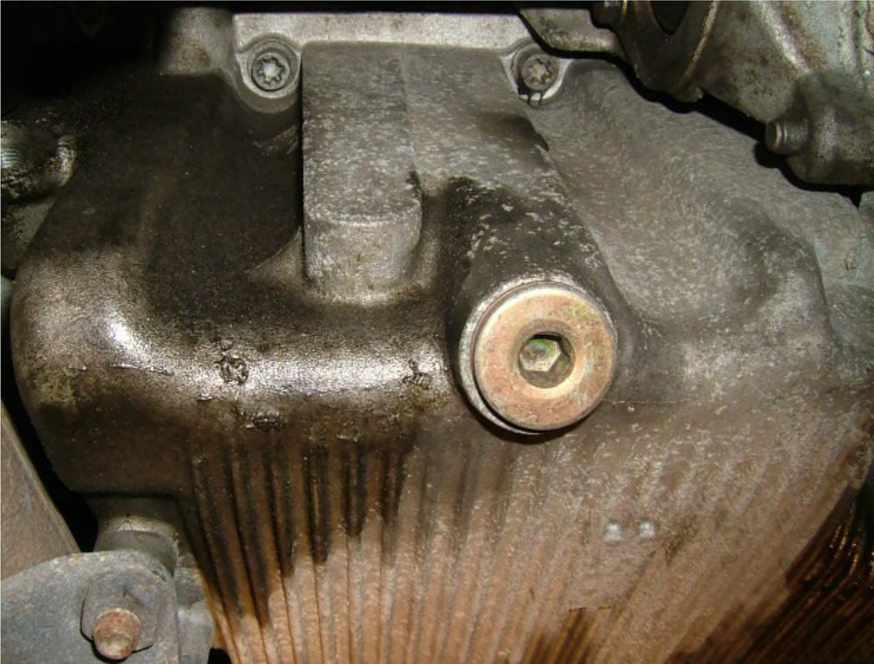
Place a suitably large basin (at least 5L) under the sump, as the next pic shows the oil flows out at an angle (not straight down) so make sure the basin is far enough back!
