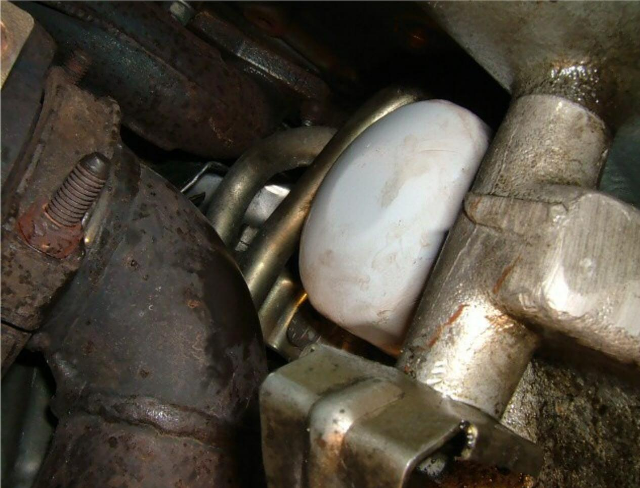
Refit the sump plug with the 8mm hex drive, but be VERY careful not to overtighten it as the thread is easily stripped!
